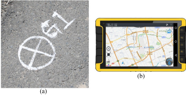
Fig. 2. (a) GCPs landmark. (b) Huace LT600T Client.
